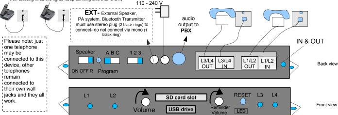
Turn the speaker ON to confirm audio is playing and adjust the volume to mid level (if device is not activated yet or it has stopped LED goes RED and there would be no audio playback - if so refer to Quick Start & activation sheet or P7)
