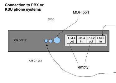
PBX phones have a **control box** with a MOH jack with telephones at each desk all connected to that control box,
