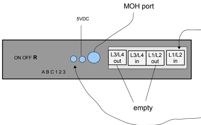
PBX phones have a **control box** with a MOH jack with telephones at each desk all connected to that control box,
